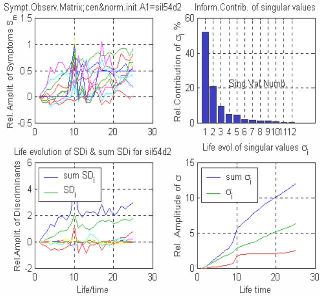
Fig. 2. The information contents of symptom observation matrix for a Diesel engine **sil54d2**, and independent fault indices  $SD_1$  ,  $\sigma_1$  as discovered by SVD.
